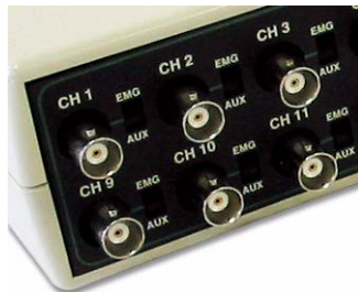
Figure 3. BNC Auxiliary Inputs. Notice the slide switch next to each BNC connector.
