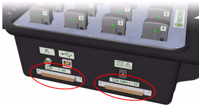
Figure 17. Analog Output connections.
