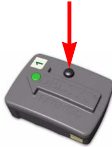
Figure 6. Turning the Trigno Sensor "ON".
